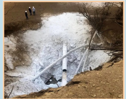
A CO 2 pipeline rupture in Santartia, Mississippi in February 2020, released 30,000 barrels of liquid CO 2 and led 200 people to be evacuated and 45 people to seek medical attention
