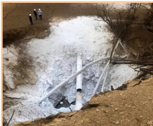
A CO 2 pipeline rupture in Santartia, Mississippi in February 2020, released 30,000 barrels of liquid CO 2 and led 200 people to be evacuated and 45 people to seek medical attention
